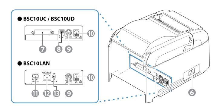
6 **Power switch** Turns the printer on and off.
