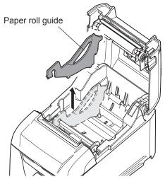
2) As shown in the figure, insert the paper roll guide in the groove.
