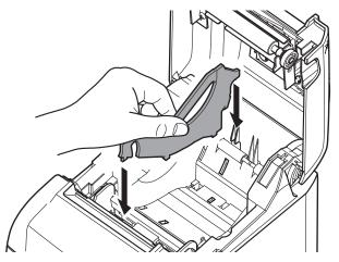
3) Secure the paper roll guide in place by pushing the section marked as "A" in the figure.
