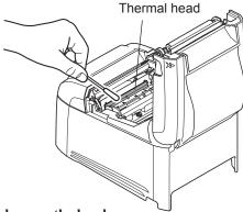
Note 1: The thermal head is easily damaged.
