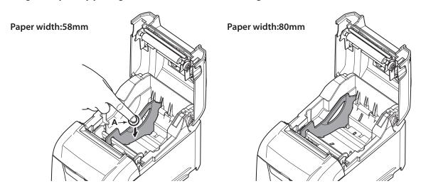
Note 1: Do not change the paper width while the printer is in use.
