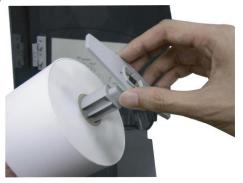
4. Place the label roll into the label roll mount. Feed the label under the carriage and over the platen.
