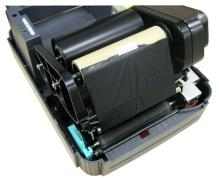
9. Rotate the ribbon rewind spindle until the ribbon overlaps the ribbon leader and stretches tight.
