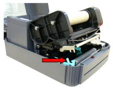
3. Slide the label supply roll spindle through the core of a label roll and attach the fixing tabs onto the spindle.
