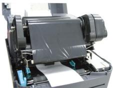
5. Adjust the label guide to fit the width of the media.
