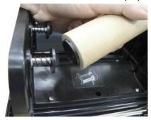
3. Please be noted that the bigger hub side with 4 ribs must be installed toward the right side of ribbon mechanism.
