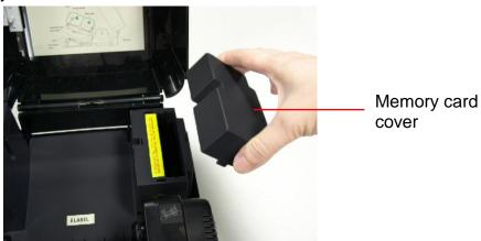
2. Plus the SD memory card module on the main board.
