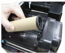
4. Install a ribbon on the ribbon supply spindle. Mount the ribbon supply spindle on the rear hubs.
