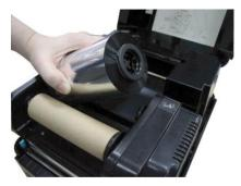
5. Insert the left side first. Please be noted that the bigger hub side with 4 ribs must be installed toward the right side of ribbon mechanism.
